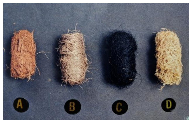
Figure 4: Cocoons made of substitute materials (A) Used fibres, (B) Jute fibres, (C) Thin plastic fibres, (D) Thick plastic fibres
